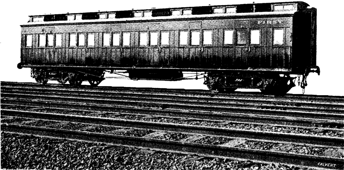
VICTORIAN RAILWAYS. FIRST CLASS VESTIBULE CAR, "AV" CLASS. (Seating Capacity, 42 Passengers ; Length over Buffers, 53 ft. 6½ in.)
